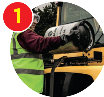
Replace empty cylinder with new full cylinder
