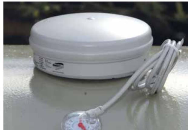
A typical tank telemetry unit
